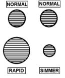
The largest pan which you should use on any burner is 230mm (9"). The base of the smallest pan should not measure less than 100mm (4").
